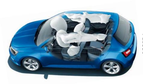
The new ŠKODA Fabia: Up to six airbags work in conjunction with five three-point seatbelts to protect occupants in a collision.
